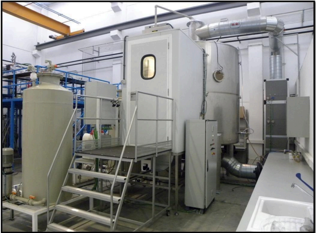
Figure 2. Image of the airtight, self-cleaning nano-exposure chamber.
