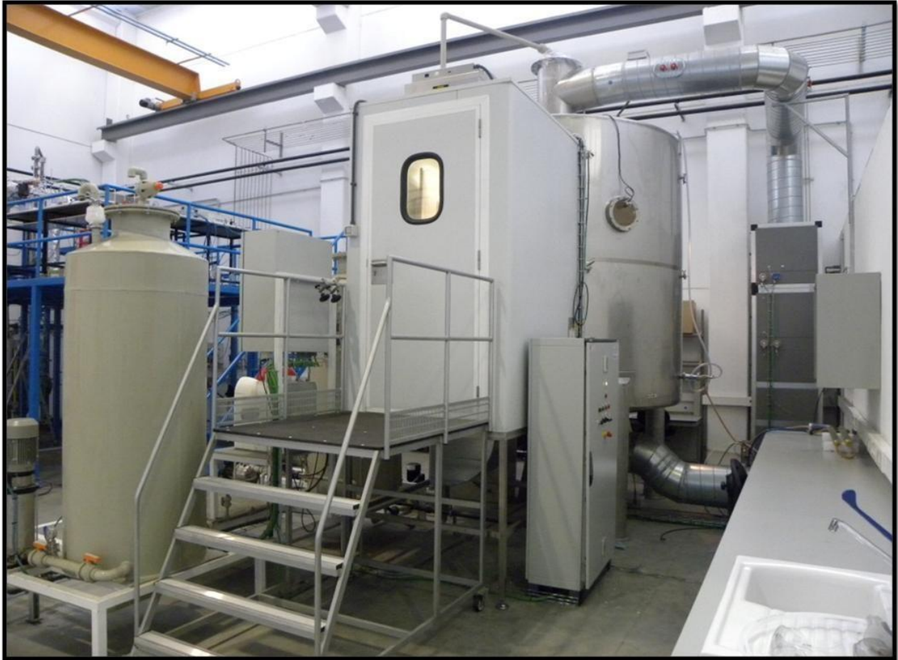
Figure 2. Image of the airtight, self-cleaning nano-exposure chamber.
