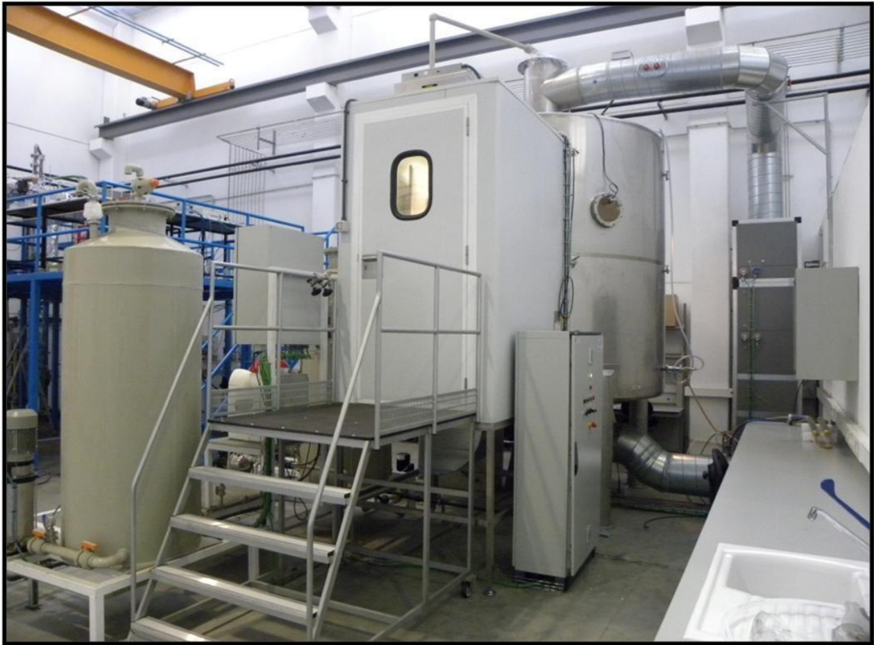
Figure 2. Image of the airtight, self-cleaning nano-exposure chamber.
